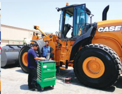
Final Engine Diagnostic Testing
